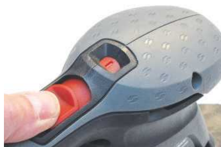
The fixed speeds are activated by a 3-way slider button
